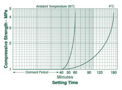
After the product has set, a minimum **curing time of 1 hr** must elapse before returning to service.
