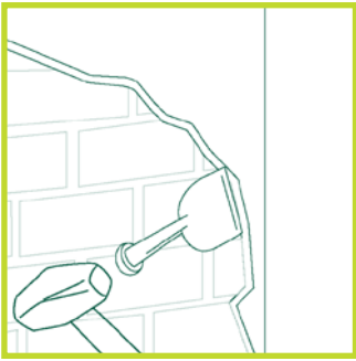
Prepare surface, remove paint, coatings, renders and plaster.
